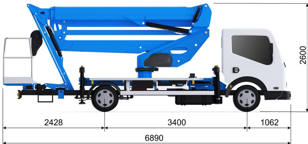
Reduced height in driving condition : 2600 mm
